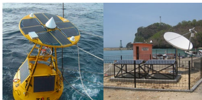
Tsunami early warning system
